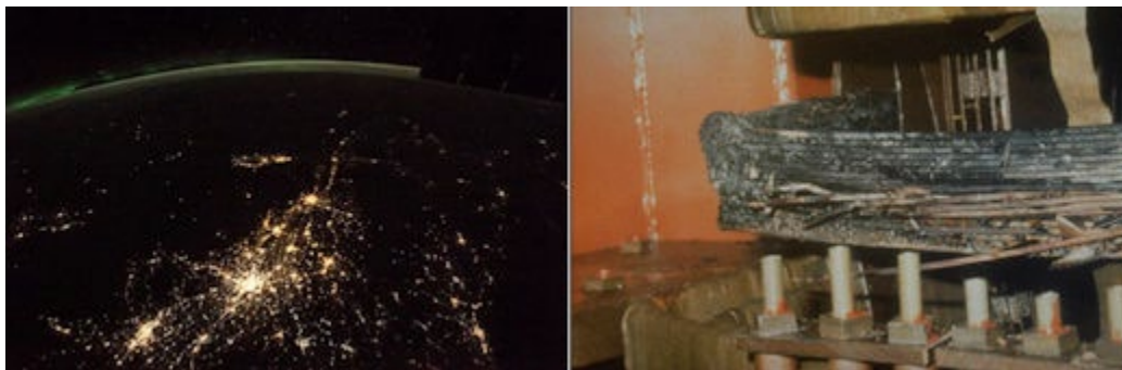
A power blackout (left) and transformer damage (right) during the March 1989 storm.
