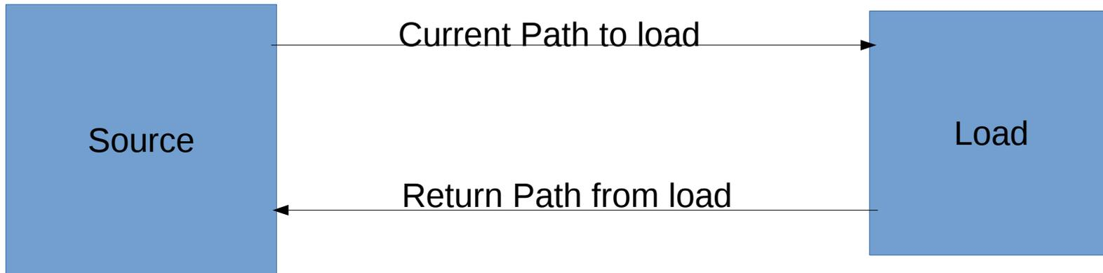
This block diagram shows a source of current, a current path to a load to make this current do something and a return current path from the load back to the source. This complete circuit is always present. Blocks usually contain components that are used for current management.
