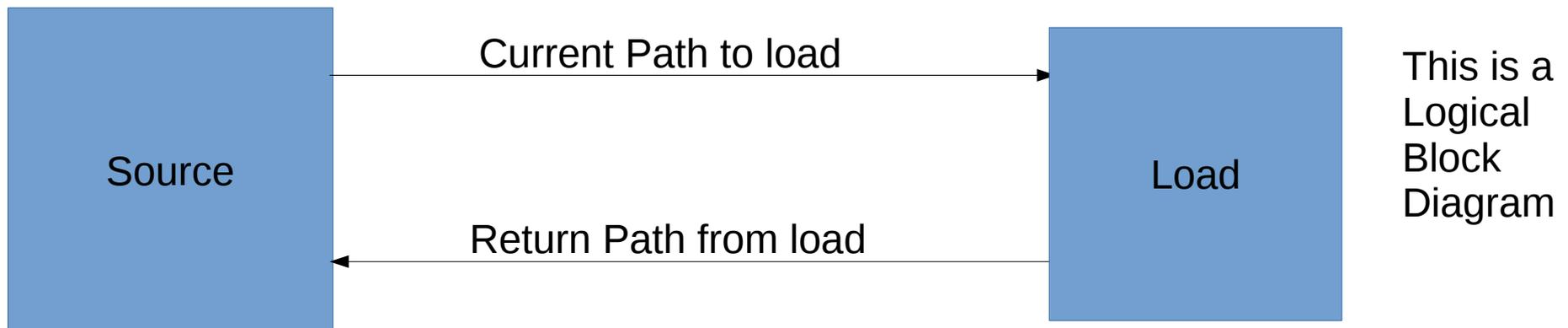
Complex Electrical assemblies are easier to understand when you break them into simple circuits with a logical block diagrams. A logical block diagram lets you label a block and or describe a function for each block without actually understanding what circuits might be in the block and the connecting conductors.
