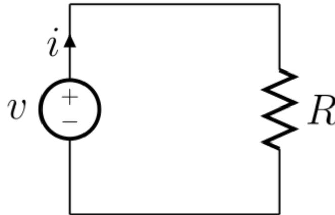
This could have been displaying an AC source and Ohms law still applies there just wouldn't be any polarization in the drawing.
