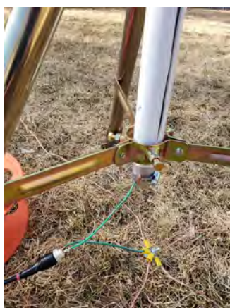
The first iteration of the feedpoint and ground plane. This 4-wire ground plane is always attached and can be used for quick setup
