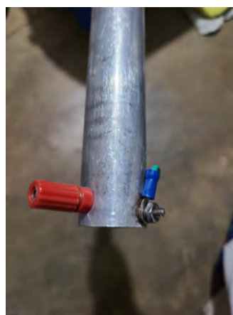
Updated feedpoint for easy deployment and quick disconnection due to weather concerns
